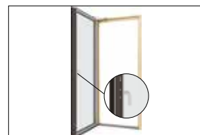
Espagnolette with handle operated brake. For all espagnolettes. Can hold the casement door in any open position from approx. 10-85°.
